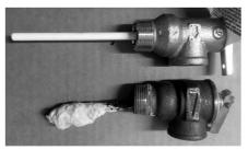
This photo compares a new T&P Valve (above) with one with sediment buildup insulating the temperature probe.
